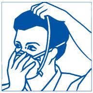
3. Pull the top strap over your head resting it high at the top back of your head. Pull the bottom strap over your head and position it around the neck below the ears.
