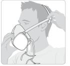
1. Place the respirator over the mouth and nose and fit the head straps as shown in the illustration.
